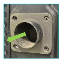
Remove the rubber gasket.
