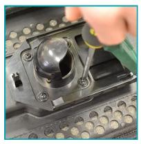
Lay the machine on the floor and undo the 4 screws surround the vacuum bag holder using a crosshead screwdriver.
