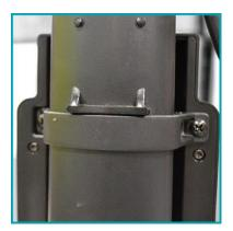
Please note that the battery clamp is currently positioned beneath the lug on the handle duct.
