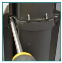
Unscrew the 2 screws in the battery clamp.
