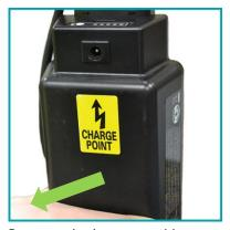
Remove the battery and battery clamp.
