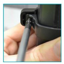
Secure the battery clamp to the latch by screwing the 2 screws.
